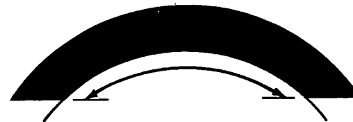
ARC LATCH DESIGN: Broad area contact with locking surface.
